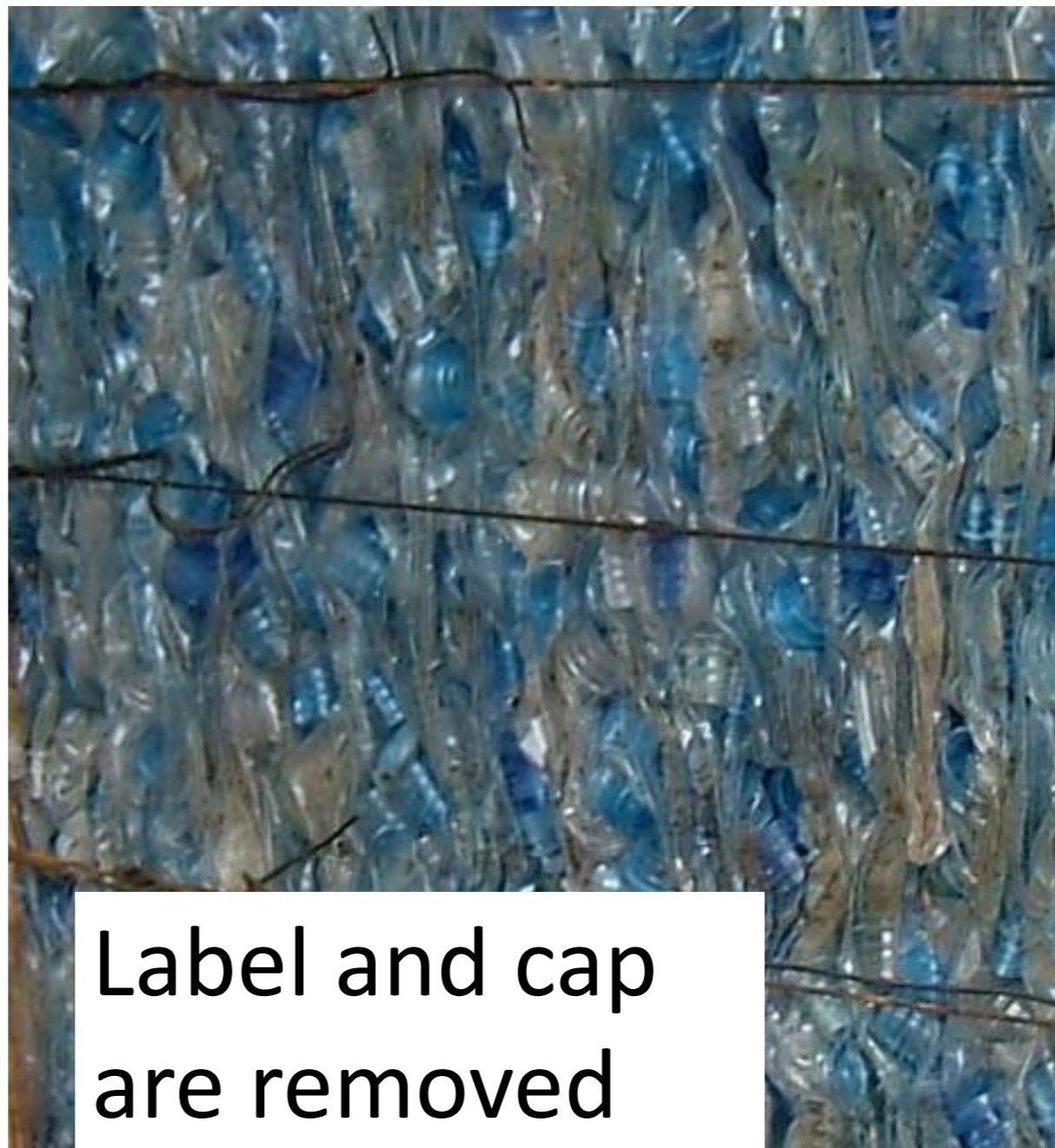
PET flake after washing and Crushing
